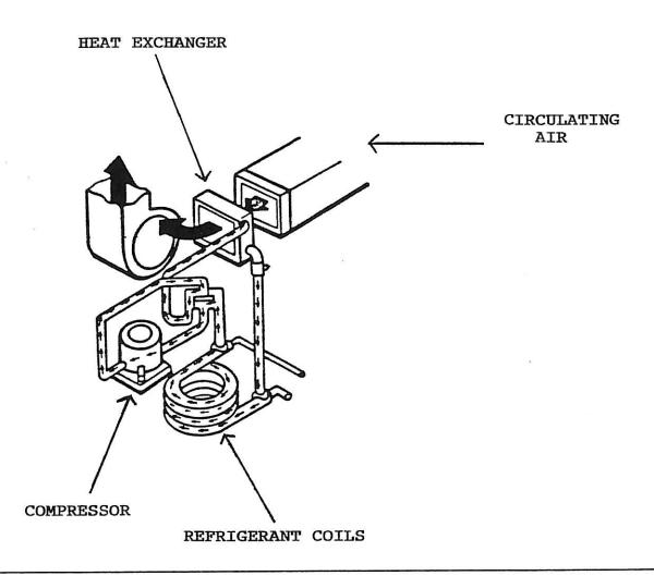
The refrigerant vapor draws heat from the air or water source. The refrigerant is then pumped to a compressor. Compressing of this gas causes it to heat itself to a temperature as much as 200°F. The hot gas then flows through a second heat exchanger where it gives up much of its heat and turns back into a liquid. Fans and ductwork direct the heat throughout the house.
